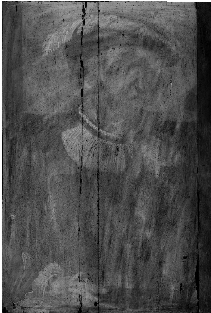
Synchrotron-sourced X-ray fluorescence mapping, lead peak
