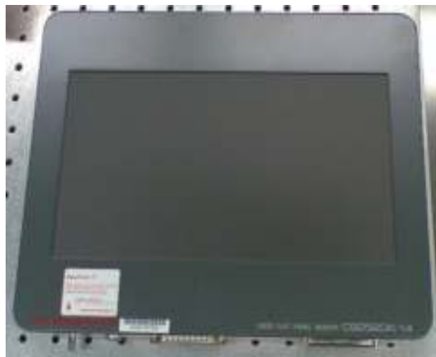
Flat-panel CMOS imager – CsI
