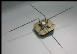
10 mNLP – multi Needle Langmuir Probe
